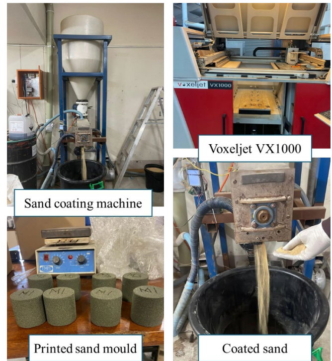
Figure 3. Laboratory equipment and materials used in this study included the sand coating machine, coated sand, printed sand moulds and 3D printer.
